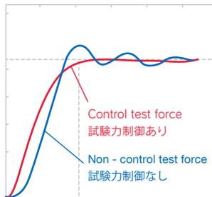
Test force is controllable with high precision from the output of a load cell.
